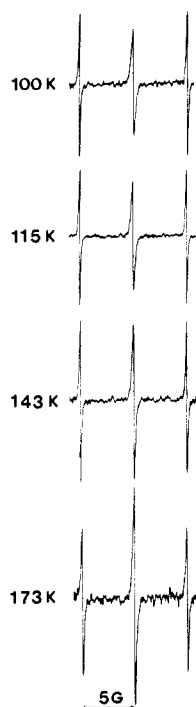
Figure 4. Low-field triplet in the EPR spectrum of the oxiranyl radical in Freon 11 at different temperatures.
